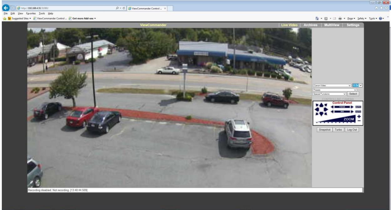
ViewCommander-Edge has a few features in its web interface that the normal version of ViewCommander does not. The Live Video page gains a “Turbo” button, which allows users to temporarily speed up video if the ViewCommander-Edge is slowing it to conserve bandwidth.
