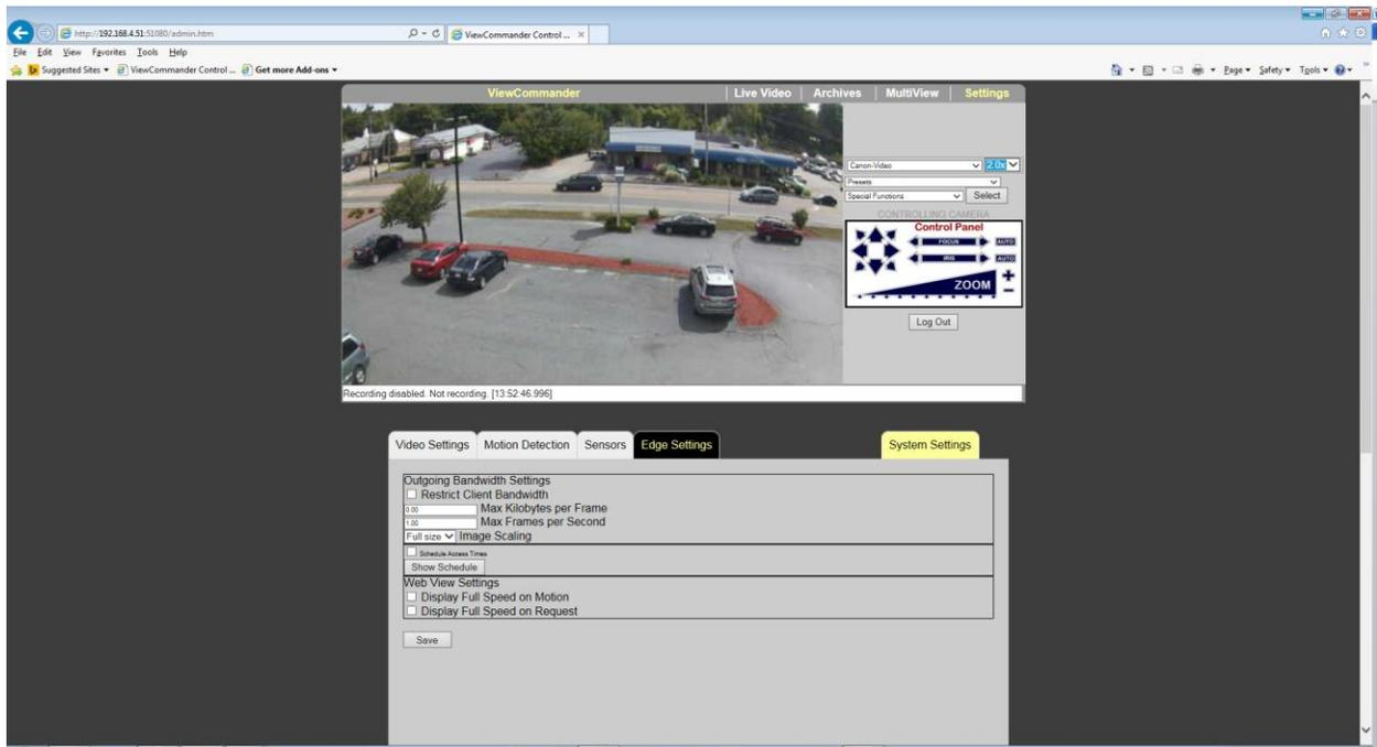
These settings, also accessible in ViewCommander itself on the ViewCommander-Edge, allow users to restrict bandwidth use, limit access times to the system itself, and configure ViewCommander to transmit video at a higher framerate either when motion is detected or on demand.
