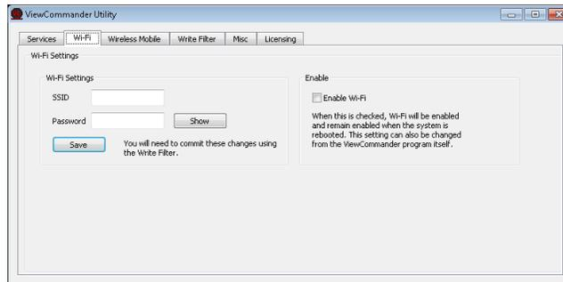
Enter a desired network name (SSID) and password, then check “Enable Wi-Fi” and press Save. Note that changes to the SSID and Password need to be committed to the Write Filter to persist after a system reboot, but changes to the Enable Wi-Fi check box do not.
