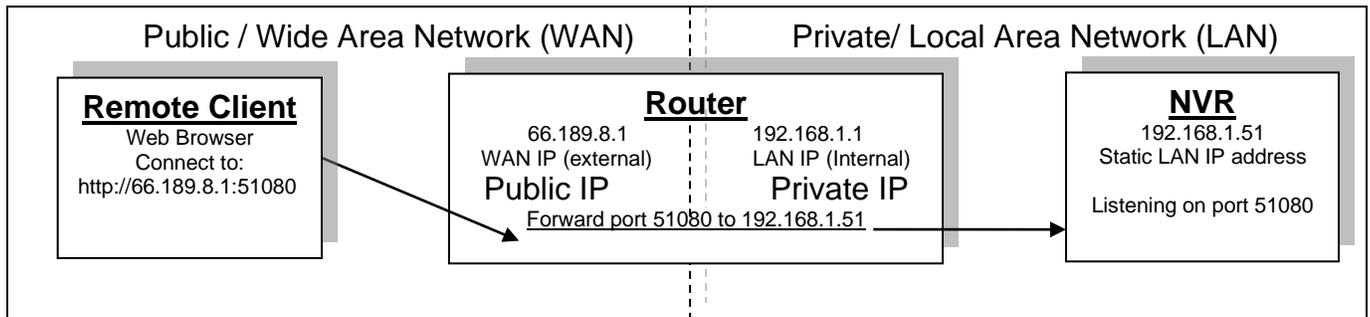
**Remote Client** – This is an application on the client computer (PC, laptop, mobile phone) such as a web browser. The client in this example is a web browser used to connect to the NVR.
